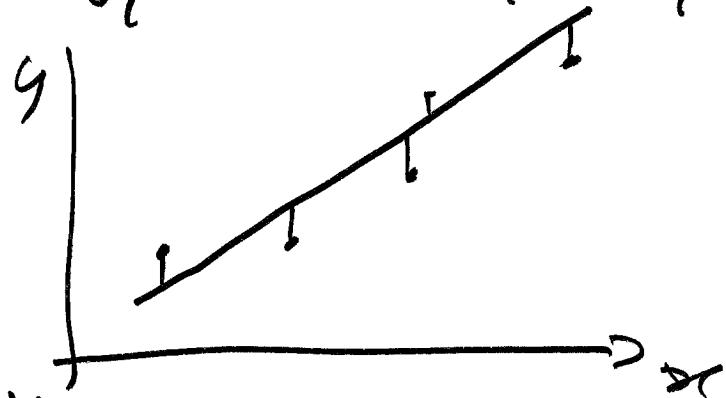
$$\sum_{i=1}^n [y_i - (a + b x_i)]^2 = Q(a, b) \underset{a, b}{\sim \min}$$
